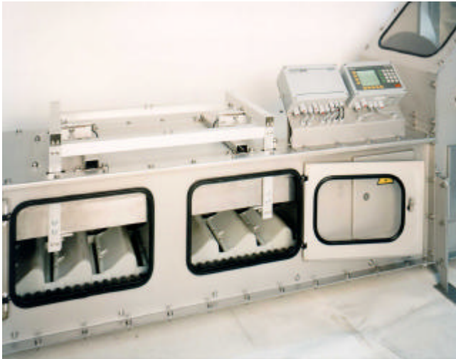
Weigh bridge, PLC control and display unit
